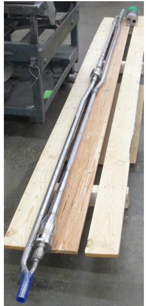
Two Stage ENO70 DOWS unit. Two ENO70 hydrocyclones and manifold piping ready for installation in drill pipe housing
