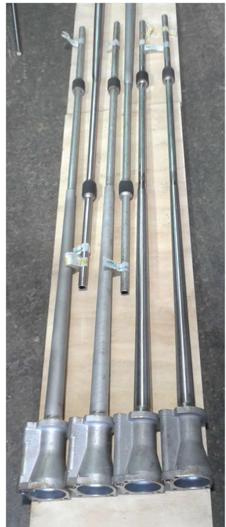
Old Generation Hydrocyclone Taper Section Supplied, with no Inlet or Reject Gallery Section
