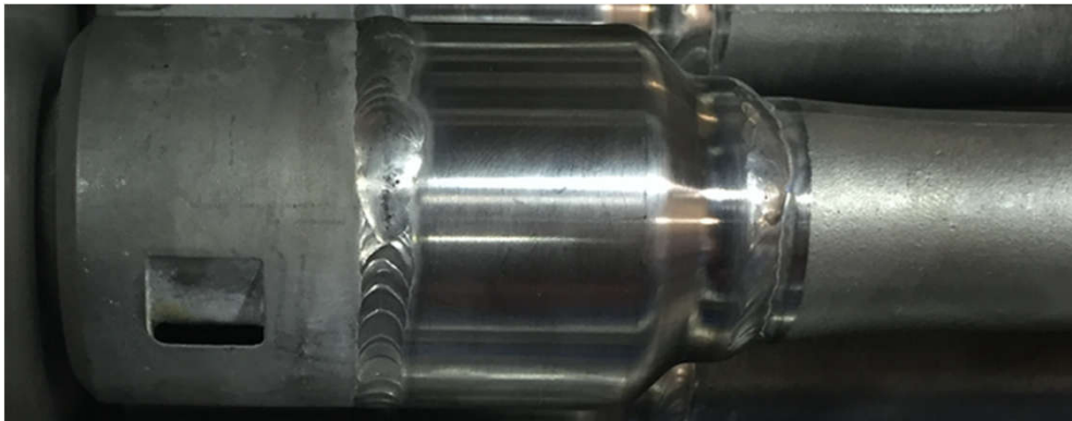
Hydrocyclone Liner with 'egg cup' Section Repair
