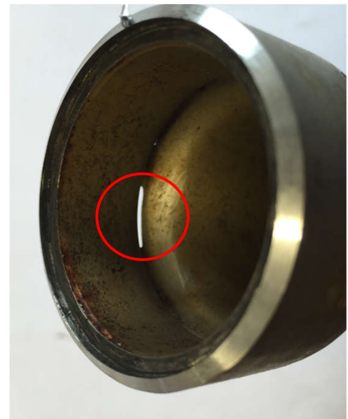
Split hydrocyclone with erosion at the top of the taper section only
