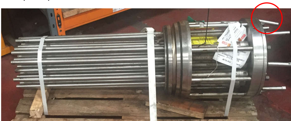
31-in-1 hydrocyclone received by EnSep ready for inspection and repair. Note damage to locating lugs circled
